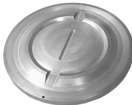
FIG. 2. Photograph of the lower electrode. Particles are shaken into the plasma; they settle into the sheath above the electrode. Due to the curvature of the sheath, they collect, forming a one-dimensional chain above the central groove.
